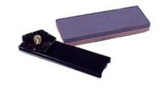
A honing guide is a jig that holds a chisel or plane iron at a constant angle against the stone. To sharpen a tool, move it back and forth on the stone to form the cutting edge. (Approximate prices: stone, \$35; guide, \$25.)
